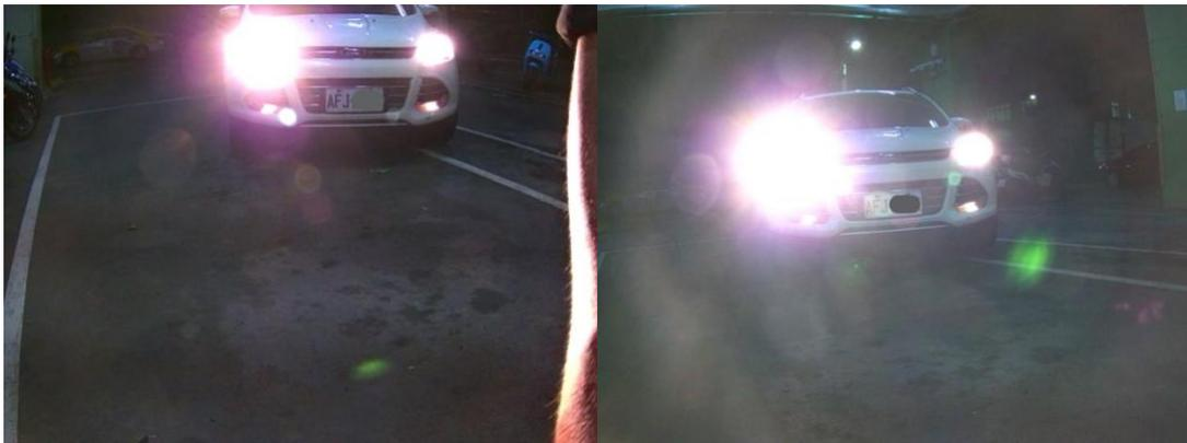
Left one is set on 1-meter height and right one is set on 0.8-meter height
