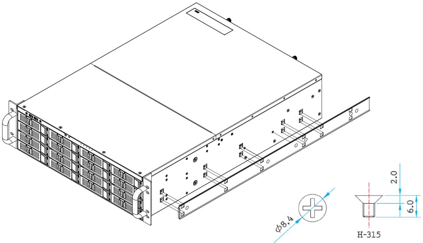
4. Insert the stag into the upper and lower square holes on the EIA rail from the back of the rail. Push the safety lock forward to secure the bracket. .
