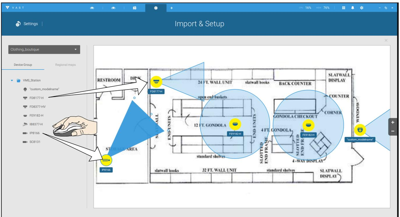
When the camera is in place, drag the FOV indicators on the edge to change the shooting angle and the coverage range.
