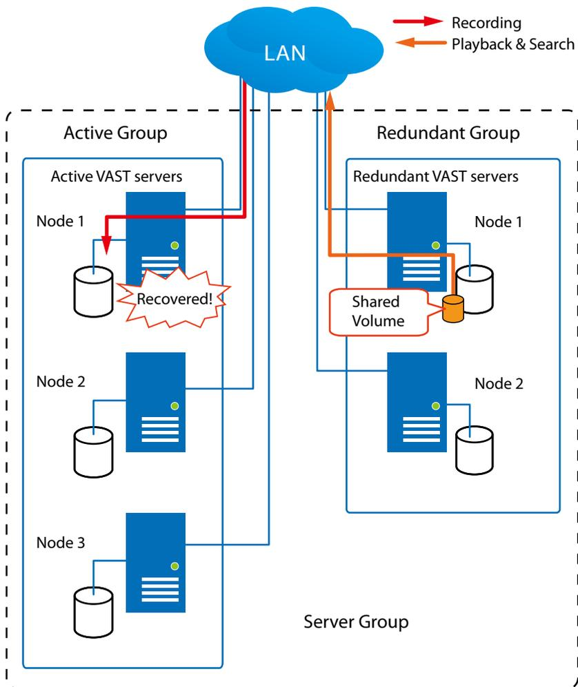
In terms of network failure, the VAST2 configuration supports Seamless Recording. For cameras equipped with an SD card, video is recorded to the SD cards in the event of network failure. Of course, the cameras must have a backup power source, such as a DC 12V input. In cases such as the only PoE switch or PoE mid-span fails, power is lost.
