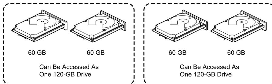
Spanning two contiguous RAID 0 virtual drives does not produce a new RAID level or add fault tolerance. It does increase the capacity of the virtual drive and improves performance by doubling the number of spindles.
