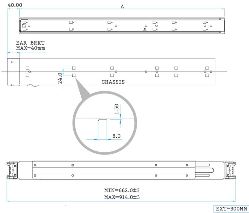
3. Secure the inner rails to the sides of the chassis using the included screws.
