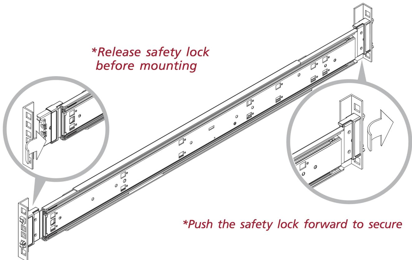
It is important to check if the safety lock is in the unlocked position before mounting the brackets.
