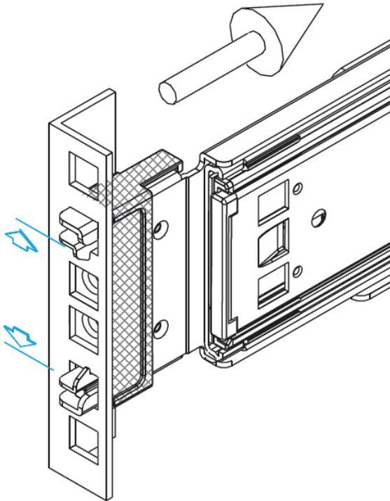
5. Lift and insert the chassis into the rack cabinet as shown below. It is important to check if the ball bearing retainer is in the fully open position before installing the chassis or it might cause catastrophic damage to the chassis if the ball bearing retainer is not in the fully open position while mounting the chassis. While you are pushing the chassis into the cabinet, you will need to release the slide from the locking position by pressing the trigger down.
