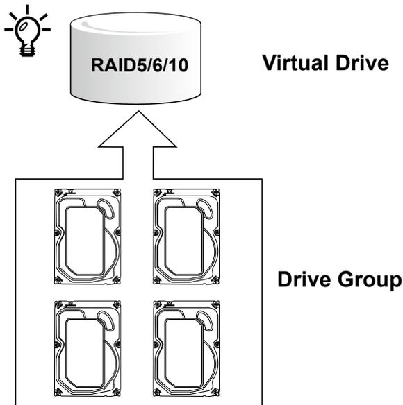
Our default recommendation is to combine 4 hard drives into 1 drive group. The capacities of these drives will be utilized to form 1 Virtual Drive. If all 16 drive bays are populated, you can create 4 Virtual Drives. A 4-member Virtual Drive can receive the video feeds from 32 cameras. You can also create two 8-member Virtual Drives to receive the video feeds from 64 cameras (CH, or channels.)
