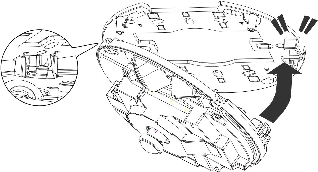
16. Install the dome cover by aligning the side-routing tab with the cabling cut-out on the base plate.
