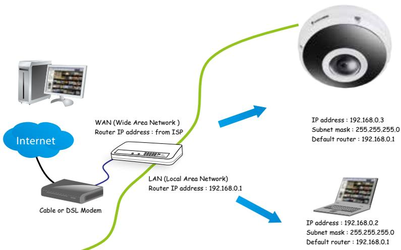
2. In this case, if the Local Area Network (LAN) IP address of your Network Camera is 192.168.0.3, please forward the following ports for the Network Camera on the router.
