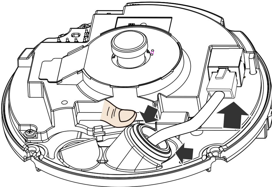
12. Pull the cable slightly backward. Please do not leave the edge of center hole folded toward the inside of the camera. Doing so will compromise its waterproof feature.
