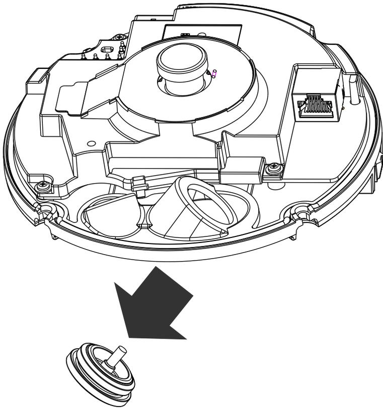
8. Remove the tip of the silicone seal by pulling it off. Insert the RJ45 connector of your Ethernet cable into the penetration cap.
