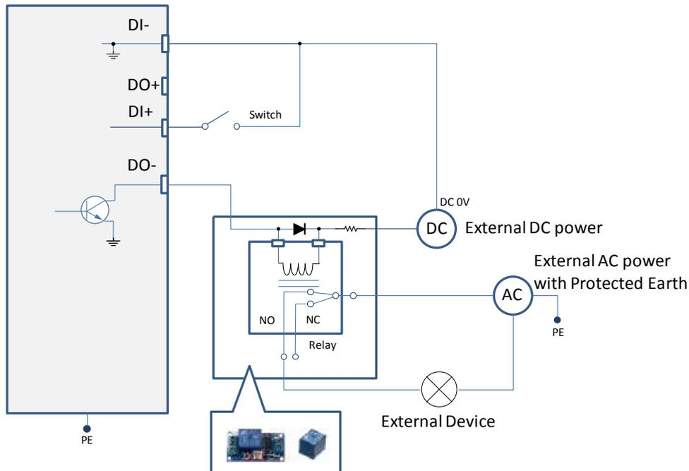
1. The DO+ pin (3.3V) provides  $3.3V \pm 10\%$  output voltages, and the max. load is 50mA.
