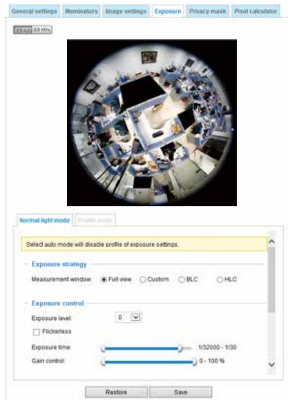
**Measurement Window:** This function allows users to set measurement window(s) for low light compensation. For example, where low-light objects are posed against an extremely bright background. You may want to exclude the bright sunlight shining through a building's corridor.
