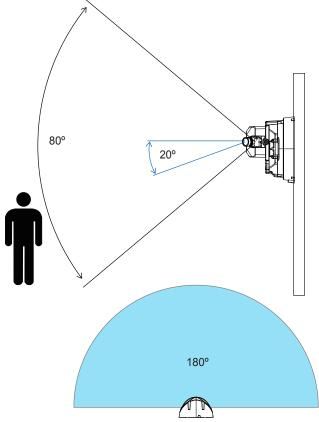
The field of view is illustrated on the left. Note that the higher the camera is installed, the larger is the blind spot area underneath the camera. The camera can be mounted at a height of 3 meters to cover a panoramic view area with its center of view aiming at the horizon. Below is the process for a standard wall-mount.
