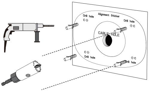
3. Hammer in the wall anchors and then install the mounting plate.
