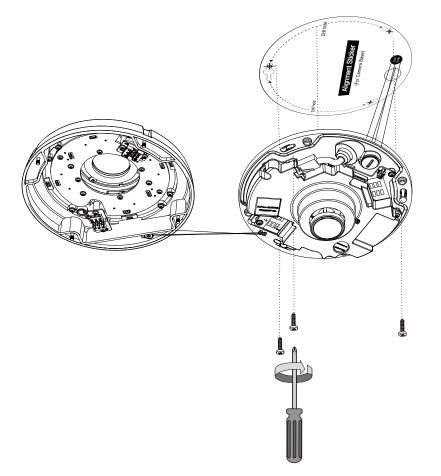
A-3. Connect the white headers of the DI/DO combo cable to the J3 and J7 headers on the camera.
