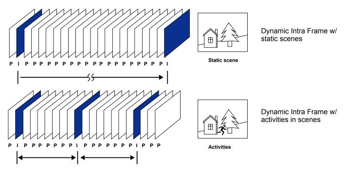
With the H.264 codec in an optimal scenario and when Dynamic Intra frame is combined with the Smart Stream function, an 80% of bandwidth saving can be achieved compared with using H.264 without enabling these bandwidth-saving features.
