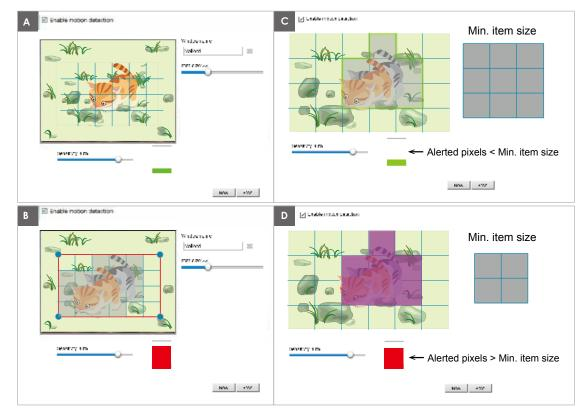
There are two motion detection parameters: Sensitivity and Min. Item Size. As illustrated above, frame A and frame B are two sequential images. Pixel differences between the two frames are detected and highlighted in gray in which the sensitivity setting will take effect. Sensitivity is a value that expresses the sensitivity to moving objects. A higher sensitivity setting allows camera to detect slight movements while a lower sensitivity setting will neglect them.
