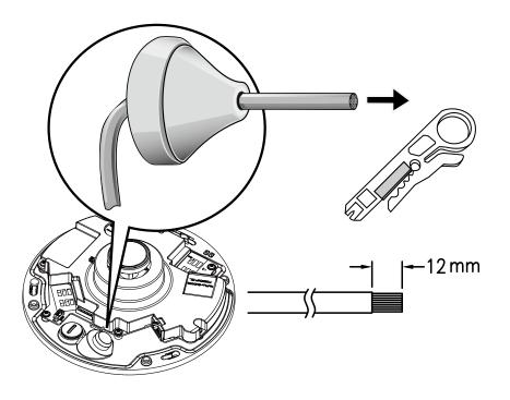
6. You will need an RJ45 crimping tool to attach the Ethernet wires to a connector. When done, connect the cable to the camera's Ethernet RJ45 socket.
