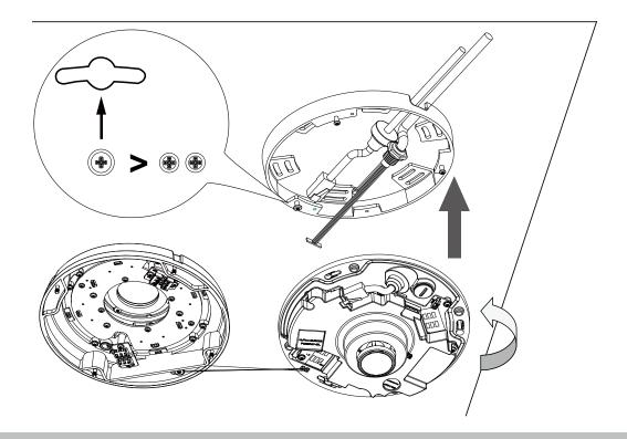
B-4. A small mount hole will be revealed through the keyhole slot. Secure the camera by tightening a flat-head screw.
