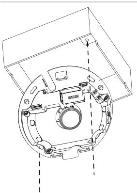
10. Arrange the cables neatly. Make sure there is a 1 cm clearance between I/O cables and the mounting tab so that cables will not get in the way when installing the dome cover.
