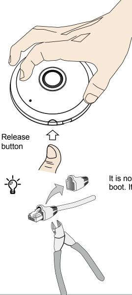
It is not recommended to use an Ethernet cable with a strain relief boot. If it does, remove the boot.
