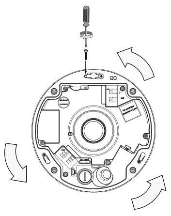
B-5. Install the dome cover using the T10 star driver.
