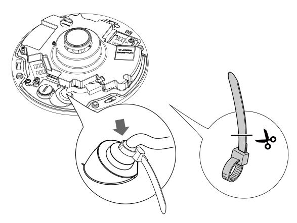
9. If the DI/DO combo cable is preferred, install the supplied rubber washer to the cable as shown in the picture. Feed the cable from the bottom of the camera and tighten the plastic nut for waterproofing.
