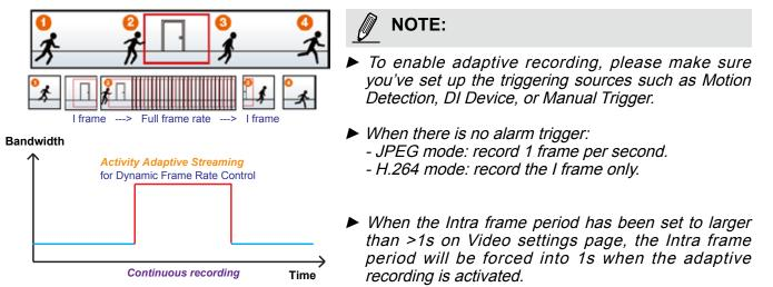
The alarm trigger includes: motion detection and DI detection. Please refer to Event settings on page 129.
