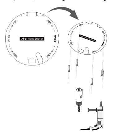
10. Secure the camera the ceiling/wall using the supplied screws.
