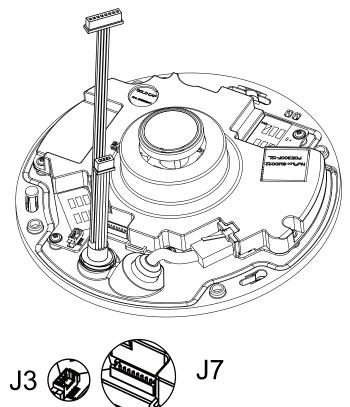
A-4. Attach the dome cover. Secure the four screws using the supplied T10 stardriver. Make sure all camera parts are securely installed.
