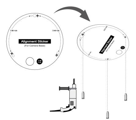
A-2. Secure the camera base to the ceiling/wall with three supplied screws.
