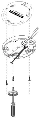
B-3. Install the camera to the mount bracket. Align the double-sided keyhole slot with the largest rivet head on the mount bracket. Turn the camera counter-clockwise as shown below.
