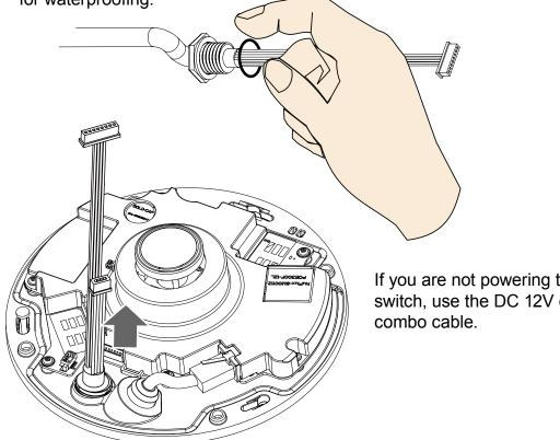
If you are not powering the camera over a PoE switch, use the DC 12V connector on the DI/DO
