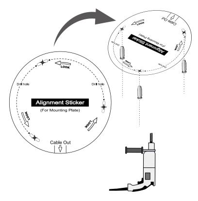
Using the three circles on the sticker, drill three holes into the ceiling. Then hammer the three supplied plastic anchors into the holes.
