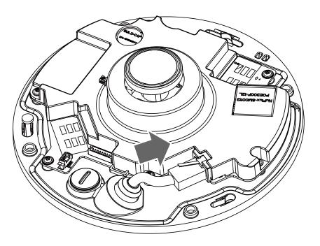
8. Use the included cable tie to fasten the top of the rubber seal so that the position of the Ethernet cable will not alter. When done, cut the excessive part of the cable tie.
