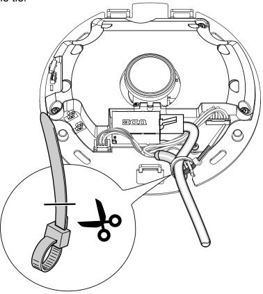
If you route cables through a drill hole on a wall/ceiling, you can simply route cables through the cabling cutout.
