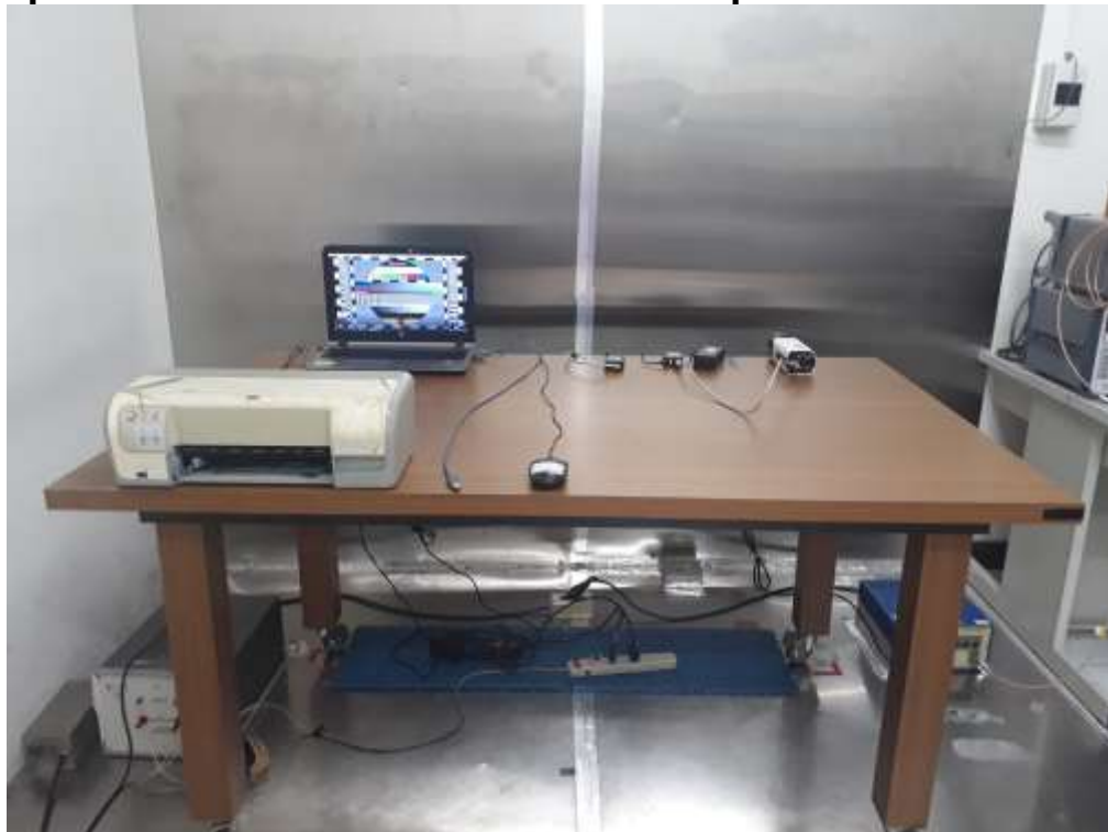
Photograph –Conduction Emission Test Setup
