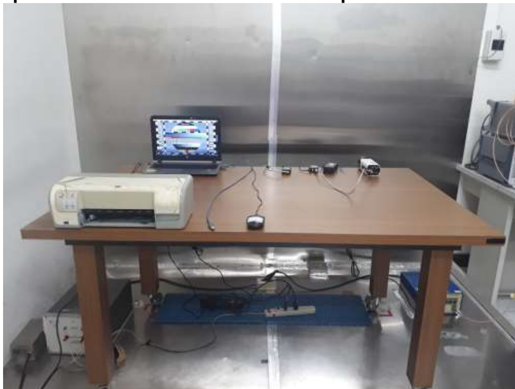
Photograph –Conduction Emission Test Setup
