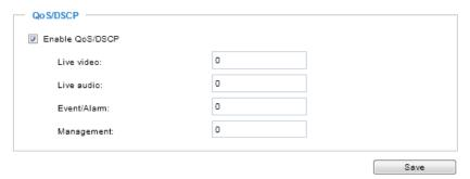
Note that different vendors of network devices might have different methodologies and unique implementations. Shown below is a sample corresponding information from a Cisco switch. You should enter a DSCP tag value according to the information provided by the network devices.
