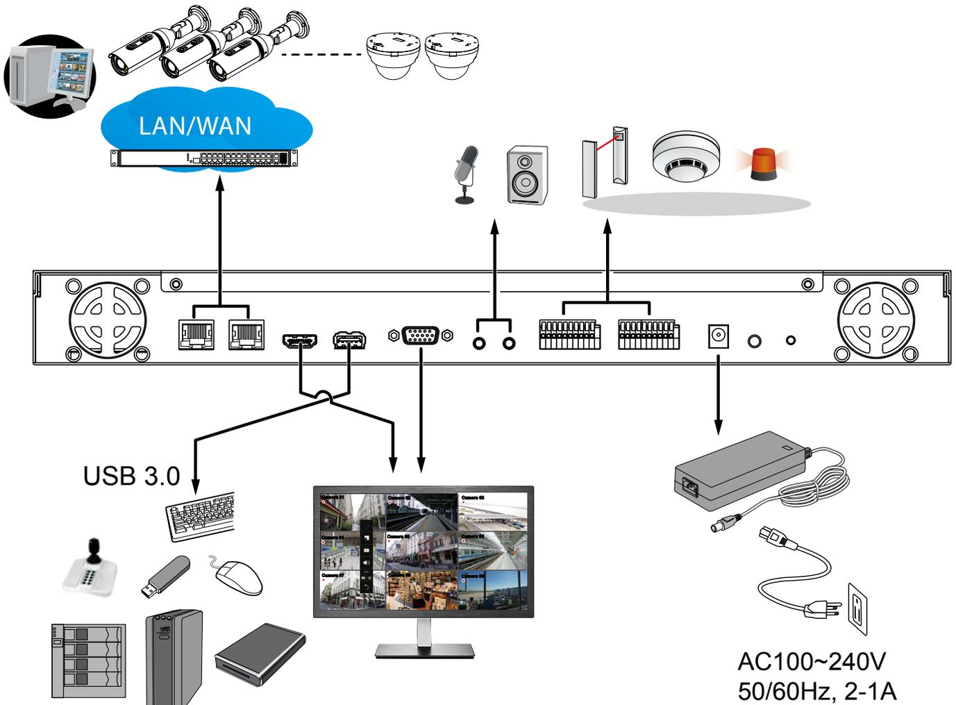
1. Connect to a monitor using an HDMI cable. VGA is also supported.
