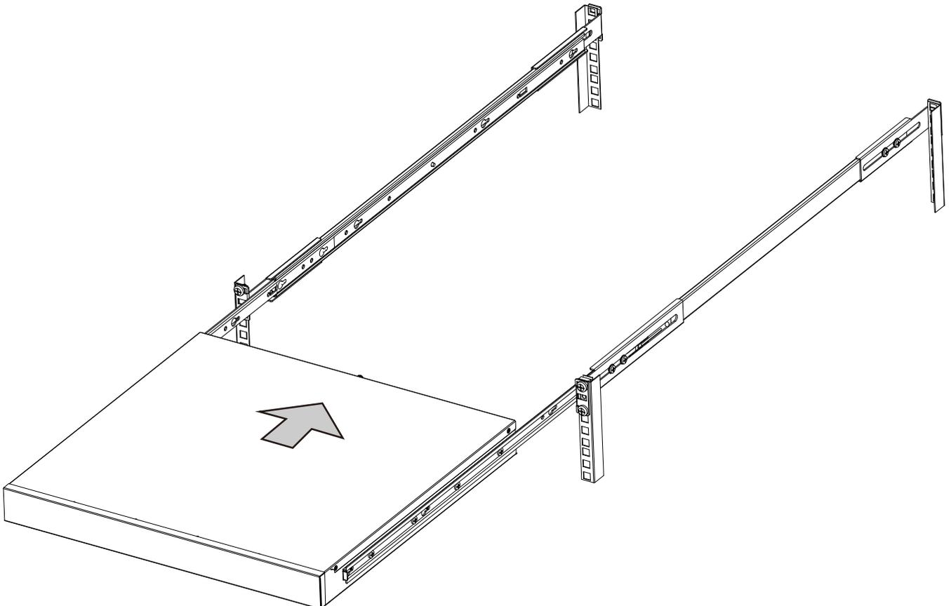
8. The inner rails and the rail assemblies should be locked on the way into the rack cabinet. Press the release tabs on the sides to slide the chassis into rack.
