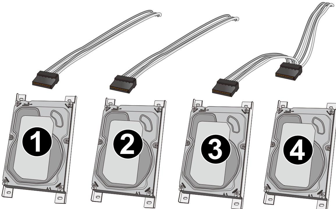
5. Secure the hard disks to the mounting positions in the chassis with its label side facing up, and the connectors facing the inside of the chassis. The sample drawing below shows the position of drive #2.
