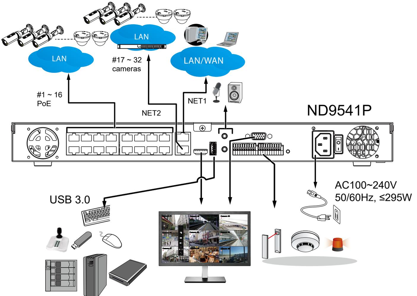
ND9541P supports 32 channel recording, and the onboard 16 PoE ports supply power and data connectivity for 16 cameras. The NET2 GbE port should be used to connect another 16 cameras in a local network via a PoE switch or mid span.
