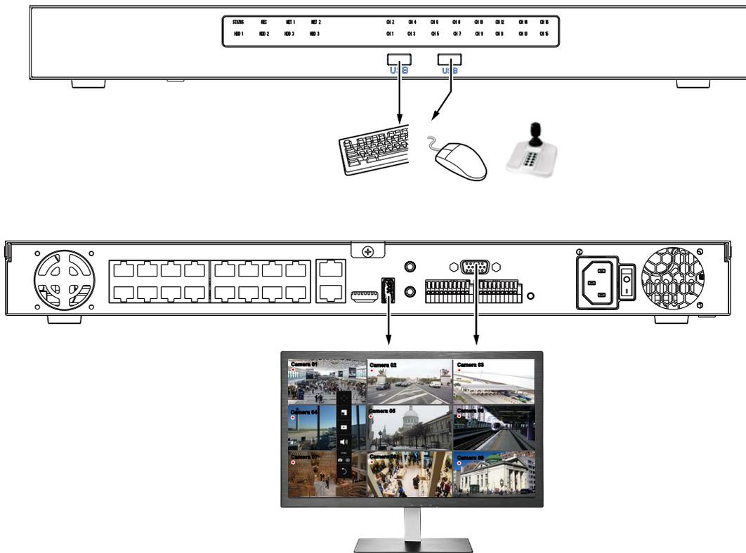
By default, a live view appears on an HDMI monitor. The interface architecture of the local console is illustrated as follows:
