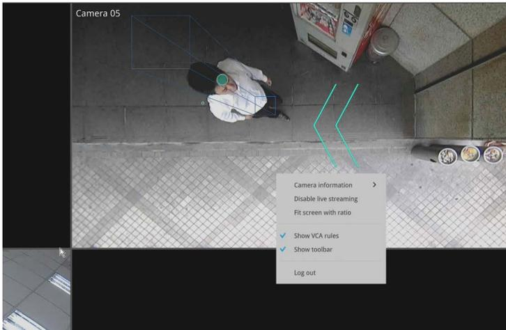
Note that the NVR supports the connection of up to 4 counting cameras. The VCA rule displays only on the 2x2 layout.
