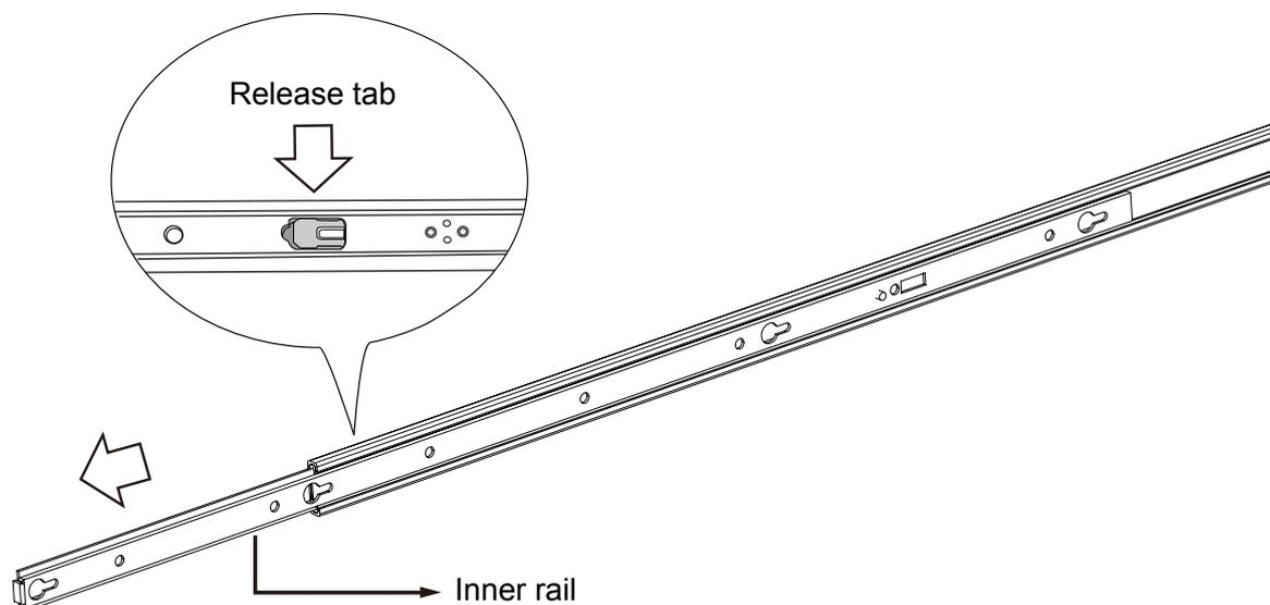
3. Secure the inner rails to the sides of the chassis using the M4 screws.
