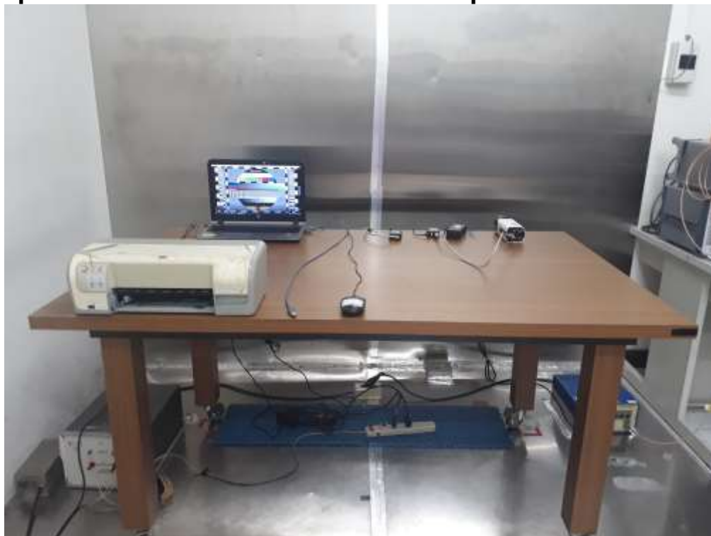
Photograph –Conduction Emission Test Setup
