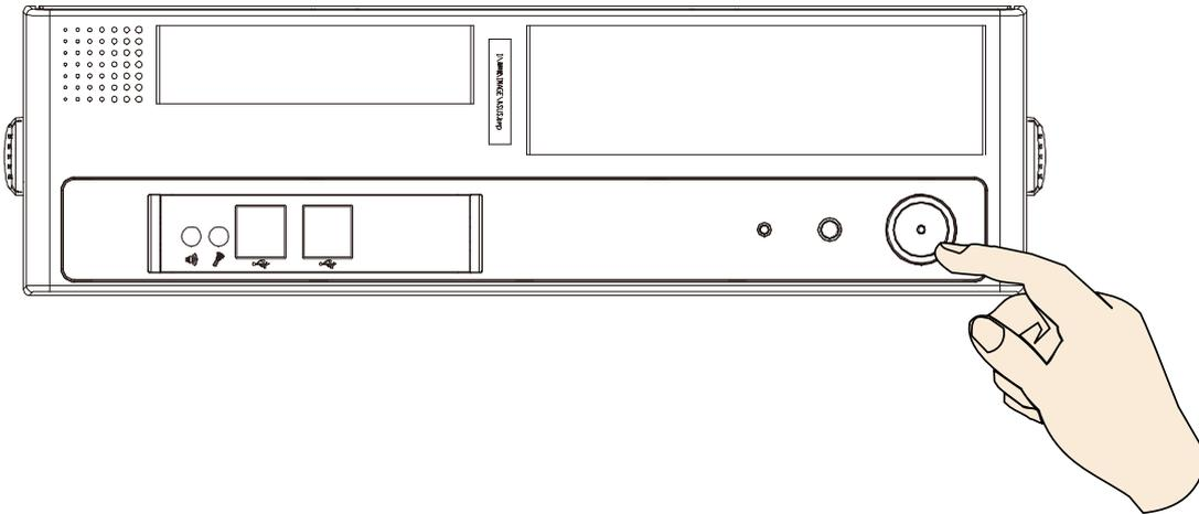
2. Skip the BIOS screens and select **Enter NVR** at the selection screen. The system will start. Wait for the start-up process to complete.
