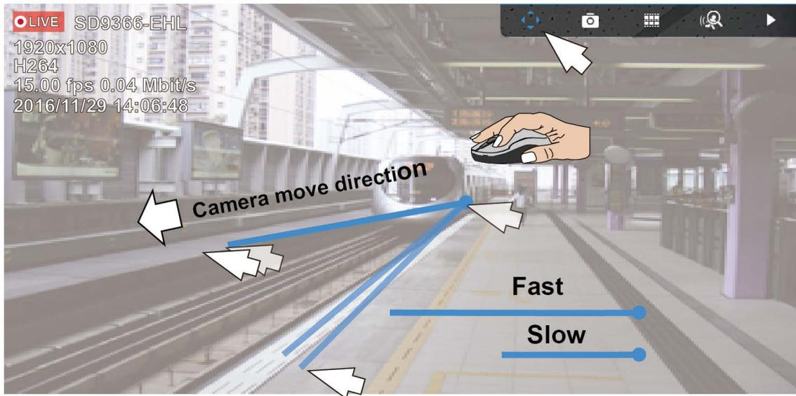
Note that while the camera is moving, you can change the move direction keeping the mouse button hold down. Release the button to stop moving.
