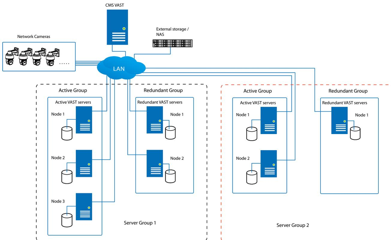
Each Redundant server can serve as the backup for ONE Active server. Depending on the number of the Active and Redundant servers, if the number of failed servers exceeds the number of Redundant servers, the failover will be abandoned. For example, if 2 Active servers failed, and there is only 1 Redundant server available, the second Active server that failed will be abandoned.
