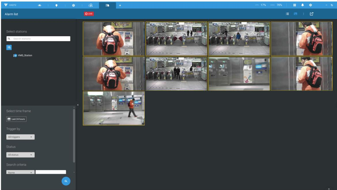
On the Alarm list, you can double-click to select a triggered alarm. A related snapshot and configuration panel will appear. An operator can select the Status menu to change the event management status. The configurable statuses can be:
