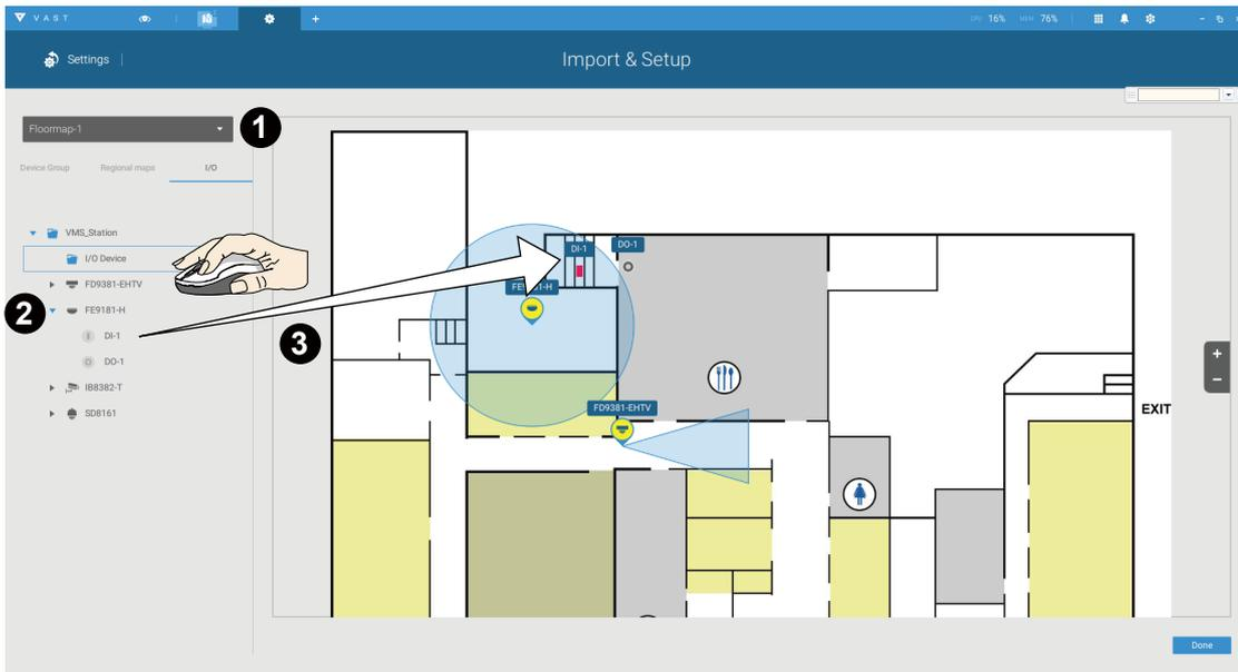
4. When a DI/DO device is selected, you can select the display colors of its icons. Configure different colors for the device status when it is normal or triggered.
