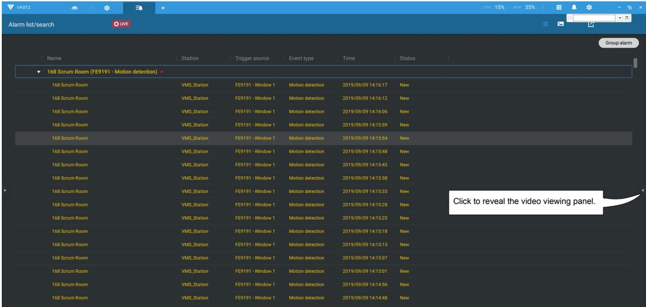
In the list mode, you can expand the right-hand-side panel. The video of the latest alarm will display.
