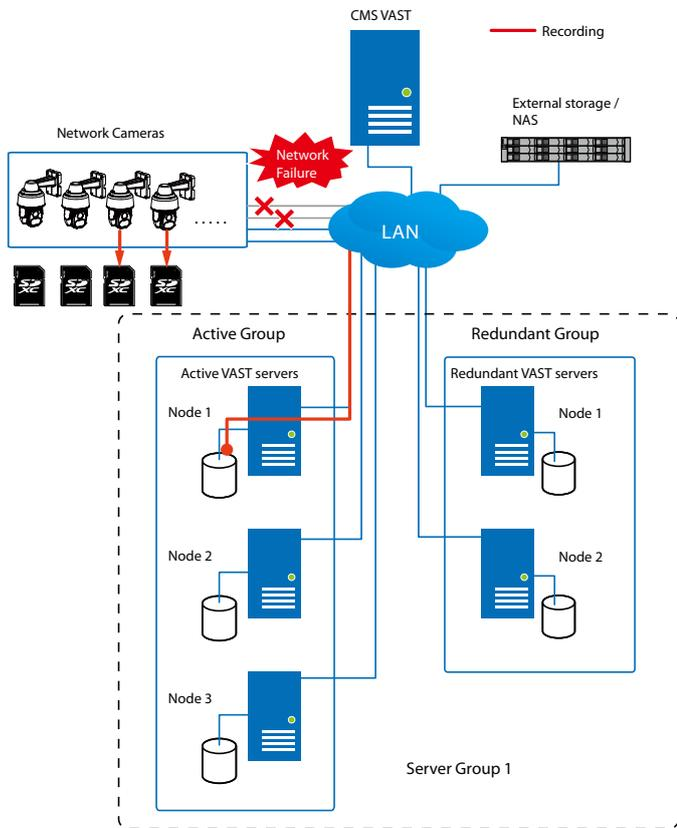
Once the network connection is restored, the VAST2 servers resume the recording task and also retrieve video segments from the SD cards. The video segments recorded during the network failure will be stitched up with those occurred before and after the network failure. The retrieval speed varies depending on the available network bandwidth and CPU resources.
