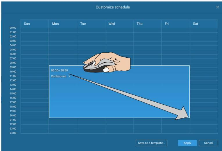
Click and hold down on the time cells, and drag the mouse to include the time span of your preference. The minimum selectable unit is half an hour. You can select separate and multiple time spans on the template.
