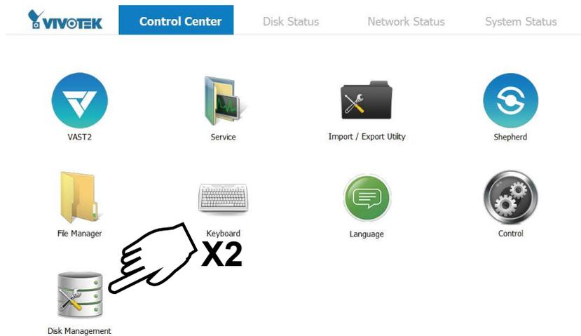
4. The hard drives you installed should appear a new disk partition Disk 1 and Disk 2. You need to initialize and format the partition before using the disk capacity. Left-click to select and then right-click to display the command menu. Click **Initialize Disk** to proceed.
