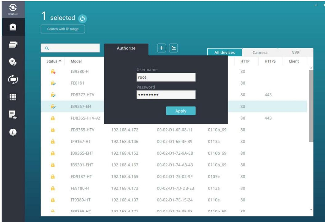
2-3-4. Make sure the selected cameras have been successfully authorized, click on the “Export device list and debug report” button. Multiple camera entries can be simultaneously selected.
