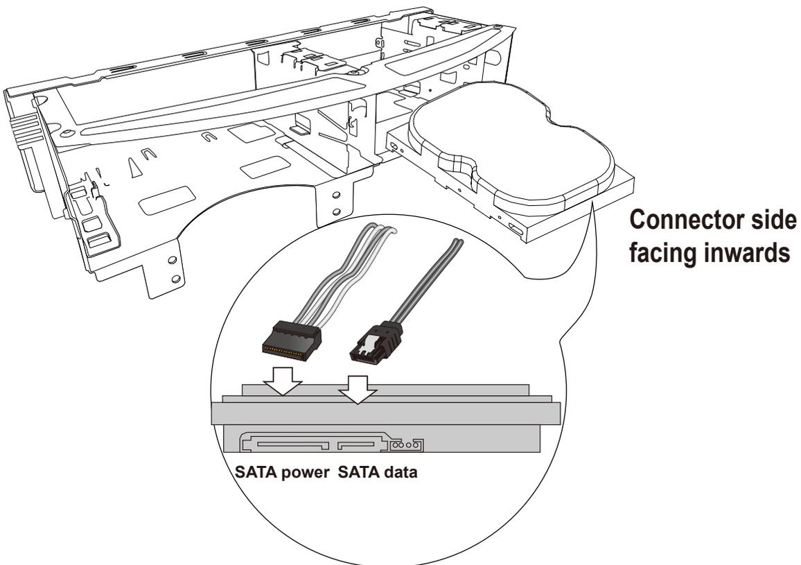
5. Secure the hard drive in the drive bay from the side of the bracket. See the through holes below.
