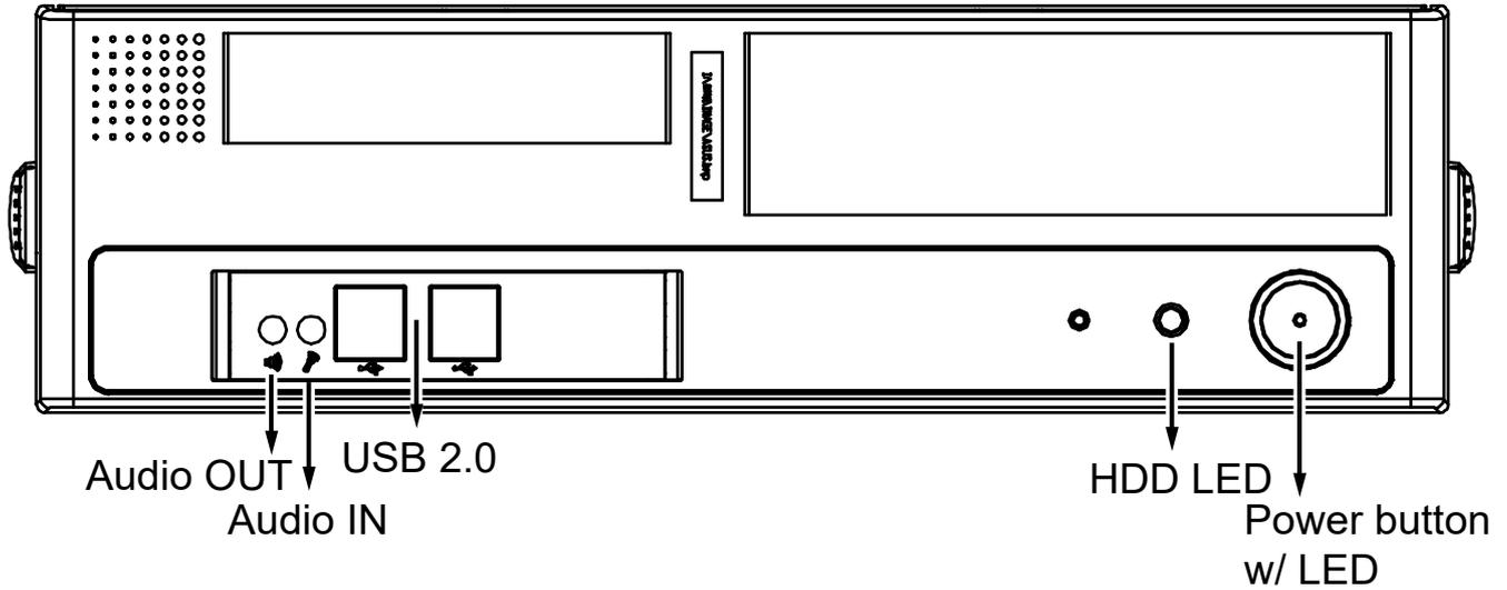
Control Panel buttons and LEDs
