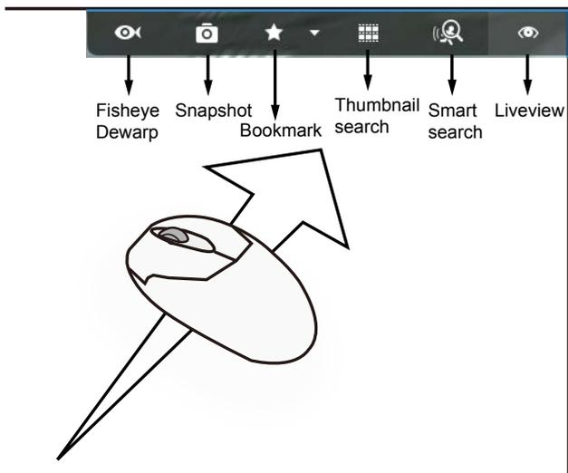
**Fisheye Dewarp:** For a fisheye camera, you can select different dewarped views during a playback. Click to select an option.
