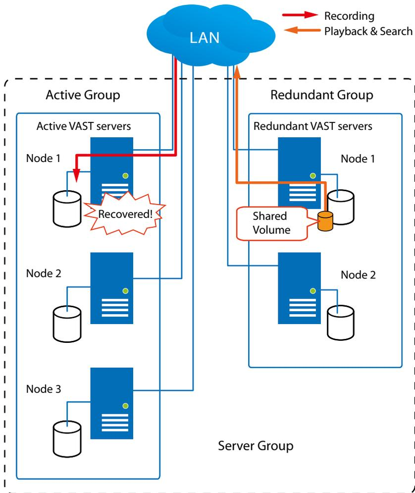
In terms of network failure, the VAST2 configuration supports Seamless Recording. For cameras equipped with an SD card, video is recorded to the SD cards in the event of network failure. Of course, the camera must be powered by a secondary power source, such as a DC 12V input. In cases such as the only PoE switch or PoE mid-span fails, power is lost.
