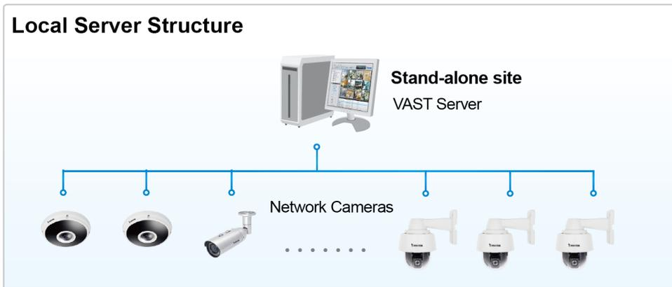
For users who manage large-scale surveillance deployments, please plan the hierarchical structure first. Then you can start to add cameras to each station and connect these sub-stations to the root station. The whole hierarchical management system is thus constructed. VIVOTEK's NVR stations can also be included as sub-stations. The Logical Tree view becomes the default.
