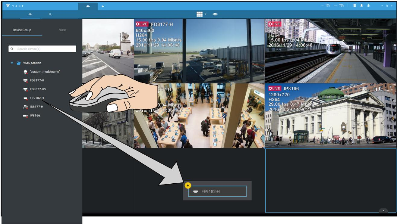
You can also fill in an Emap by dragging and dropping a pre-configured Emap into a specific view cell. Click on the E-Map tab to select a pre-configured E-Map. Note that an E-Map should be placed into a larger view cell.
