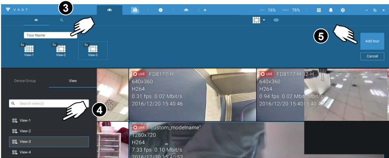
The default for the duration of the display of each view is 5 seconds. You can right-click on each view to display the Duration of each view. You can apply the same duration of all views, or allow each view to display on screen for a different span of time.
