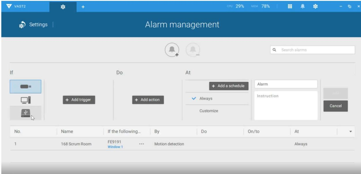
2. Select **VIVOTEK ANPR** as your triggering source. Select and create triggering conditions such as character height, image width, list, list name, country, etc. Use "=" for text matching, "~" for text containing, or approximately matching specific characters, and also ">," "<," ">=," "<=" for numbers larger or smaller than a preset value.
