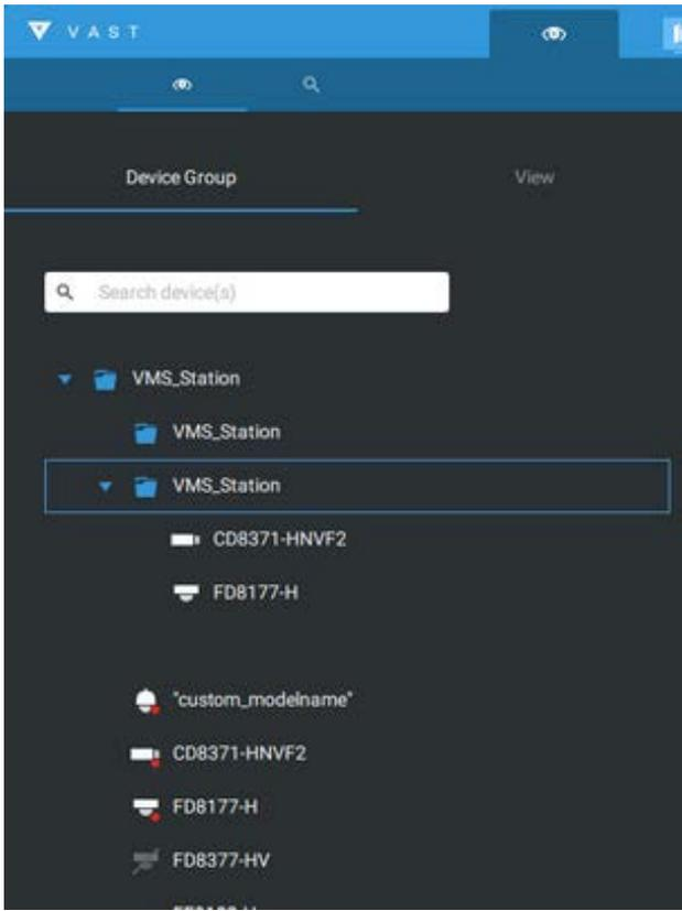
When you want to enlist an NVR into your configuration, please remember to enable the access from VAST server in the NVR's Service page. The connection between VAST and NVR is made via encrypted https. If the connection port is changed to a non-SSL port, the access from VAST to NVR will fail. For adding the ND series NVR, use port 443.
