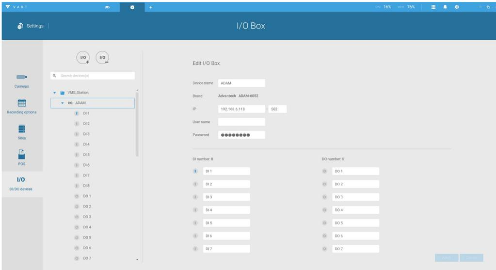
Enter the I/O box's IP address and credentials, and select the correct model name from the pull-down list on the right. Click the **Apply** button to proceed. The current I/O connections are also displayed on screen, such that the status is displayed when DI pins are connected to detection devices.
