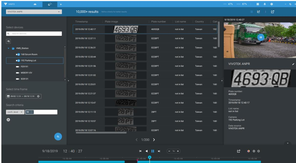
You can click and drag the display names of individual columns to switch their positions on the screen. The changes to layout are stored on the client computer. After you re-arrange the order of columns in search results, the display order will also be applied to the exported CSV file.
