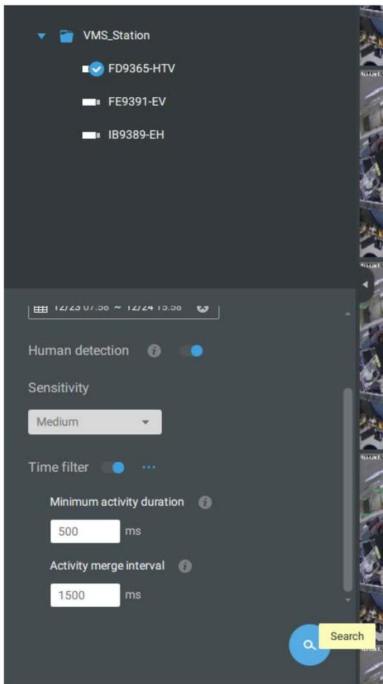
You can specify the time span, Human detection, Sensitivity level, and time filter parameters in a Smart Search II panel.
