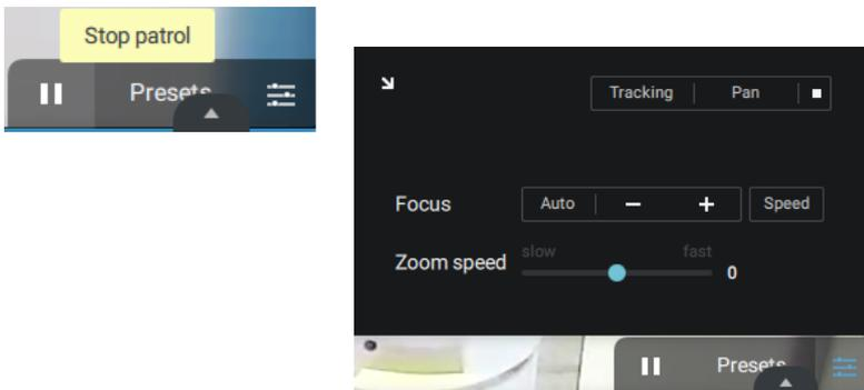
The PTZ settings tab allows you to enable PTZ Tracking and the Pan functions. You can also adjust the Zoom and Focus speed, or manually adjust the focus. Please refer to the camera User Manual for more information about these functions.
