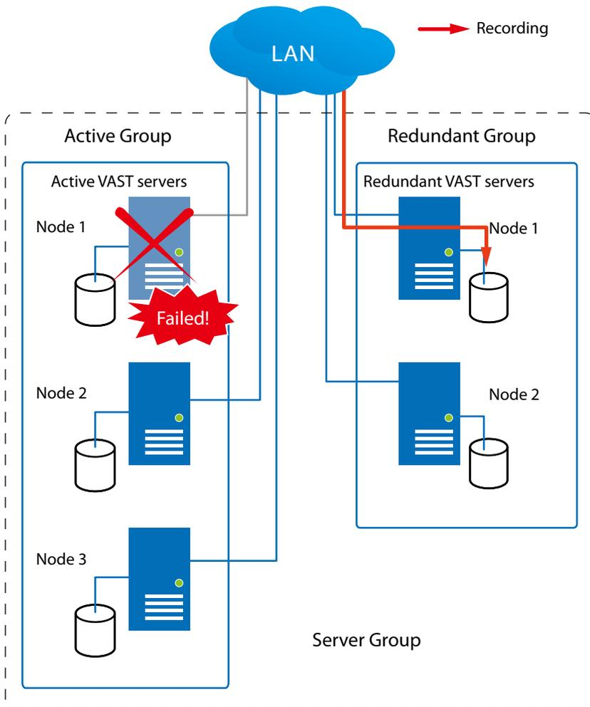
Once the server in the Active group is restored to normal operation, and a CMS server requests for the recordings and data occurred during the time the active server failed, the requests will be fulfilled by a shared volume on the redundant server. Due to the concerns with network bandwidth and processing power, the restored active server does not synchronize its recording pool with that on the redundant server.
