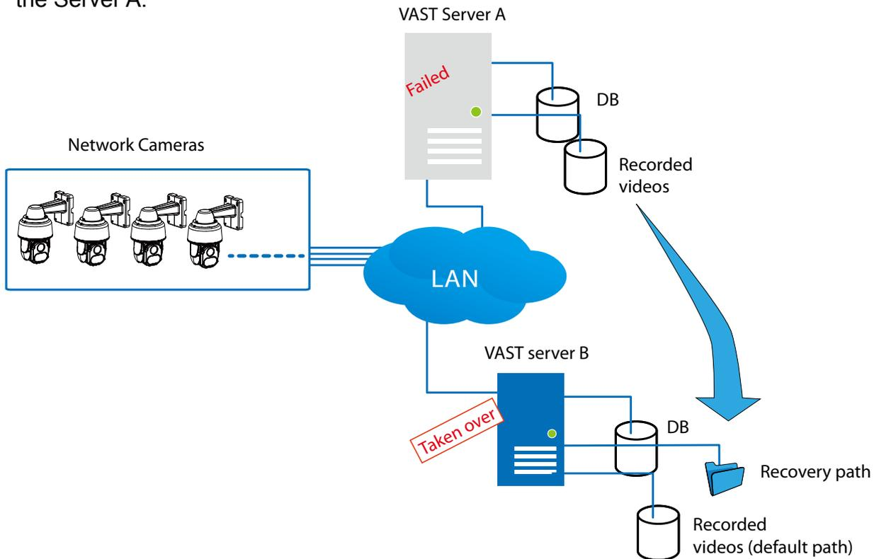
2. The VAST server B is used to continue video recording. The previous recordings on server A can be retrieved by attaching the hard disk(s) to server B or manually copying to a storage device on server B. You can then designate the location of these files as the "Recovery path" from server B. An administrator can then use the VAST software to access the past recordings.
