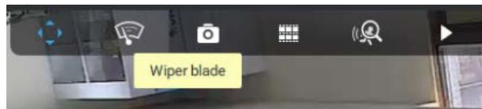
For speed dome cameras that comes with wiper blade, the wiper blade control button will be available on the tool bar.
