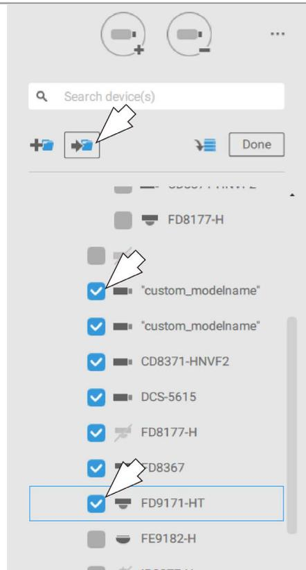
6. Select a logical folder to move the devices to. The selected devices will be listed under the logical folder you selected. Repeat the process to move cameras to each logical folder.
