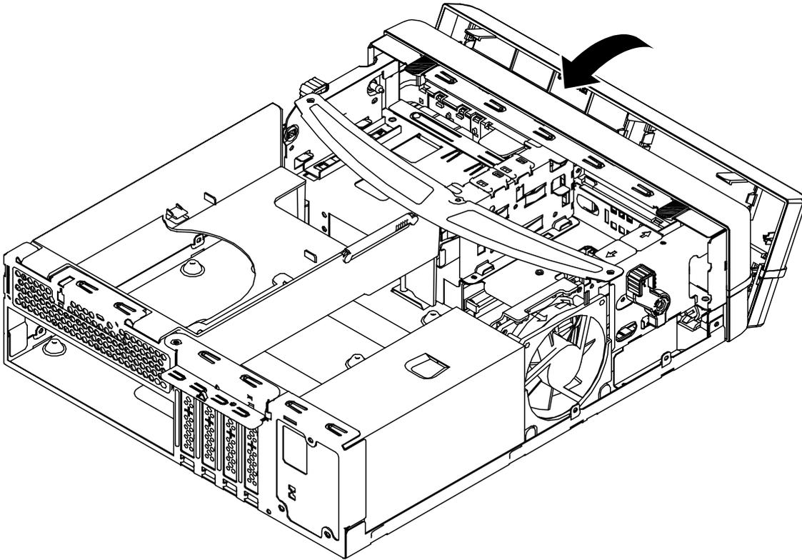
8. Install the top cover by sliding it into place and fasten the retention screws.
