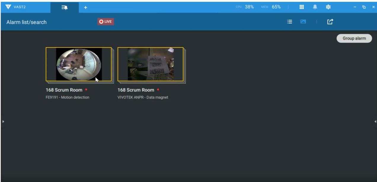
When the alarm action is set to "Send live streaming," the videos coming from the same camera will occupy only one view cell.
