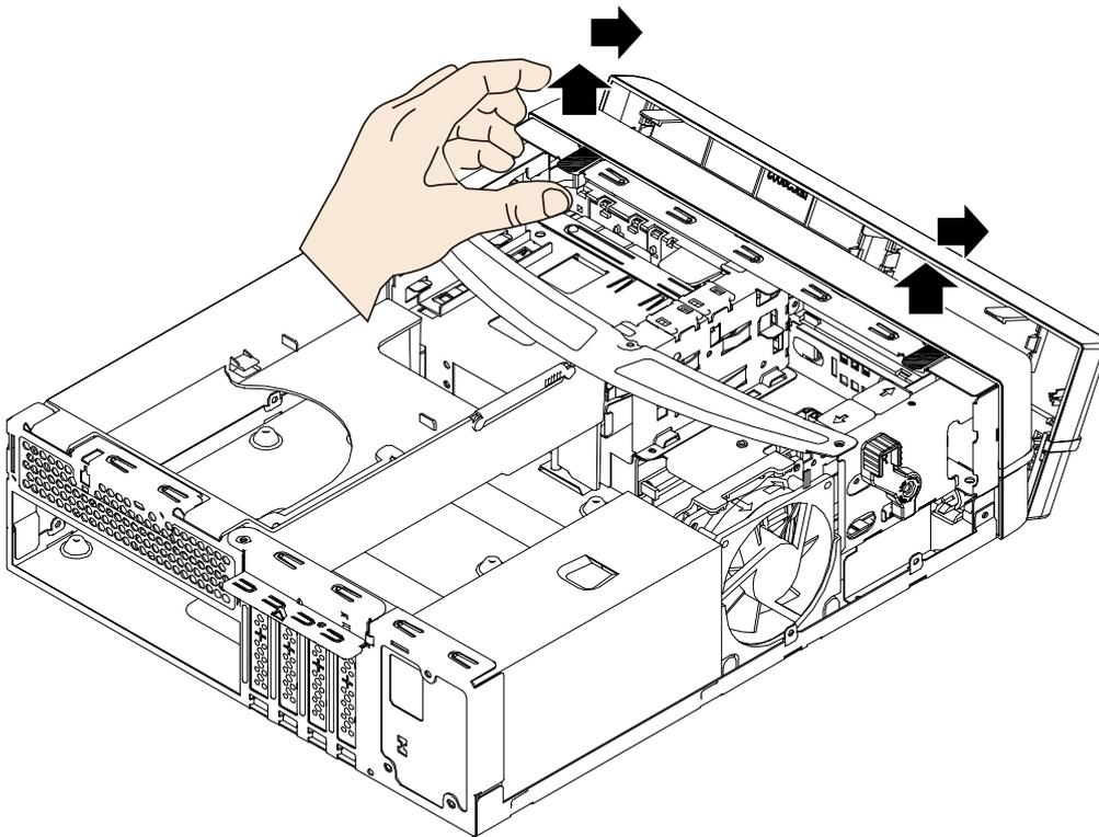
3. Pull the retention levers on the sides and remove the front section bracket.
