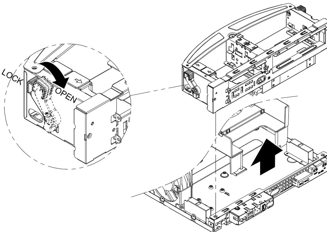
4. Install 2 hard drives to the locations indicated below: 1. under the bracket; 2. into the drive bay.
