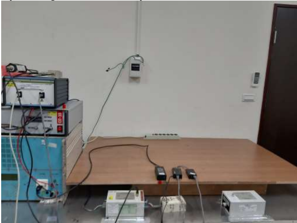
Photograph –Surge LAN Test Setup
