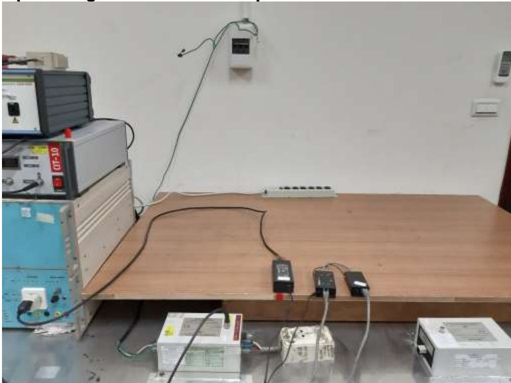
Photograph –Surge & EFT Test Setup
