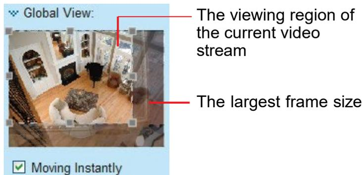
Note that the PTZ buttons on the panel are not operational unless you are showing only a portion of the full image. If the live view window is displaying the full view, the PTZ buttons are not functional.
