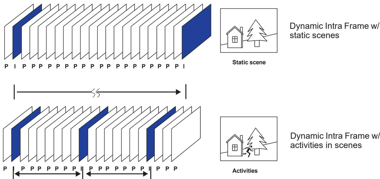
With the H.265 codec in an optimal scenario and when Dynamic Intra frame is combined with the Smart Stream function, an 80% of bandwidth saving can be achieved compared with using H.264 without enabling these bandwidth-saving features.
