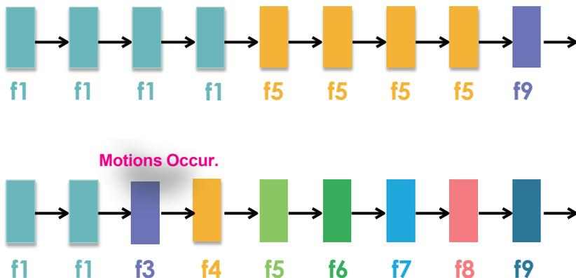
By queuing the old frames from a static scene, both the computing efforts and the size of P frames are reduced. It is beneficial for keeping up with the frame rate requirements.
