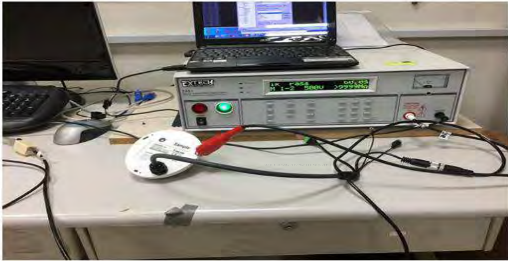
Insulation measuement test and Voltage withstand test Environment
