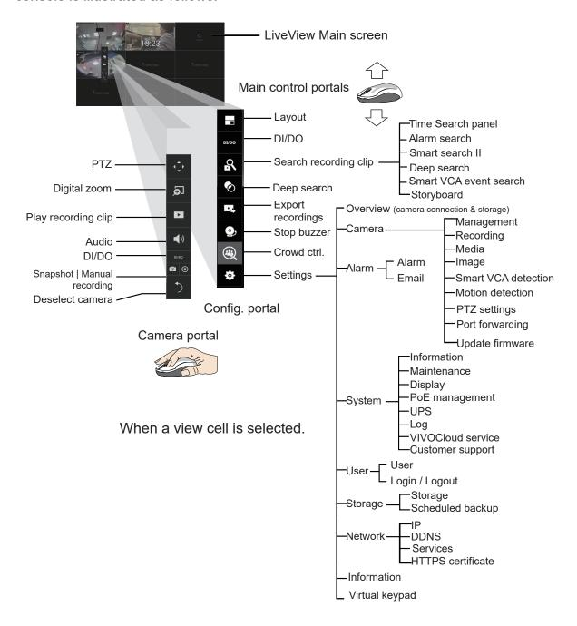
After you finish configuring using a Camera portal, click again on the camera view cell to reveal the main control portals.
