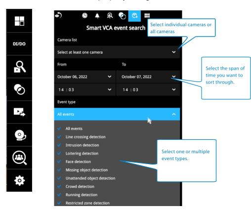
4. Click the Search button to begin the search. Depending on the scale of the search (how many cameras involved, and the span of recordings in search), the search should be completed in a few minutes.
