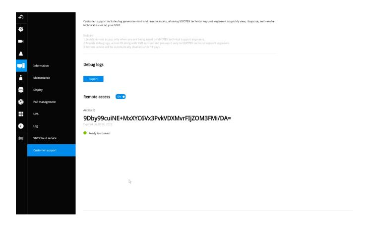
If network unavailable message is displayed at the lower screeen, the network connection between NVR and cloud server may have failed.
