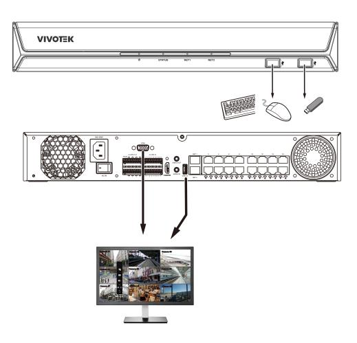
By default, a live view appears on an HDMI monitor. The interface architecture of the local console is illustrated as follows:
